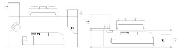
The minimum recommended air change ratio (C) must be observed to maintain the required air quality and prevent unwanted gas accumulations (refer to Section ⇒ Potentially explosive
